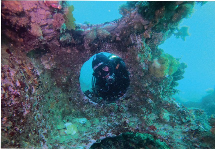
Paul Spencer looks through stern pillow block that supported propellor shaft.wreck
