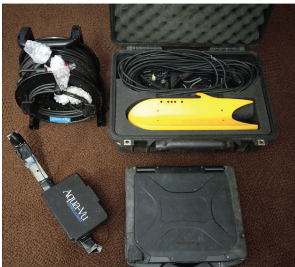
The Starfish CHIRP side scan, 50 m cable, drop camera and Toughbook computer - a compact remote sensing ensemble weighing less than 20 pounds.
