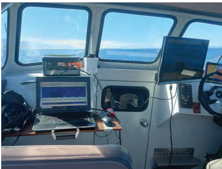
Equipment setup on one of two vessels employed during MAS's 2023 field season. The laptop is connected to the magnetometer and runs associated software, while the boat operator uses the computer monitor and an integrated GPS to drive transects
